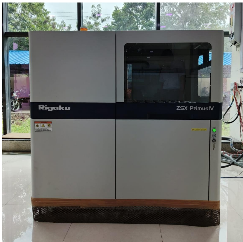
Photo - 12: Photographs showing WD-XRF instrument (Rigaku, Japan) at Chemical Lab, MECL, Nagpur
